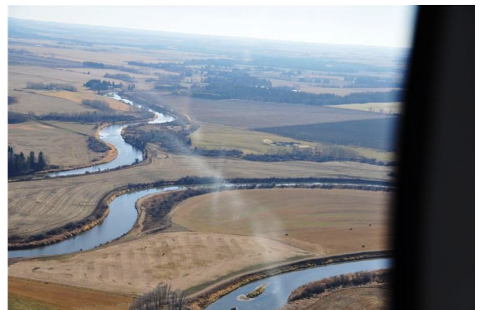
This is the area which the last gravel application was for. You can see where 6M was already gravelling out (look at the area just south of the vegetated strip). This area is subject to spring flooding at the existing elevation. You might be able to see why we think lowering it would cause a river cut across leaving the loop stranded!
